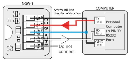
Figure 2 - PC / RS232 Port Connections
