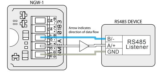
Figure 3 - RS485 / IEC 61162-2 Port Connections
